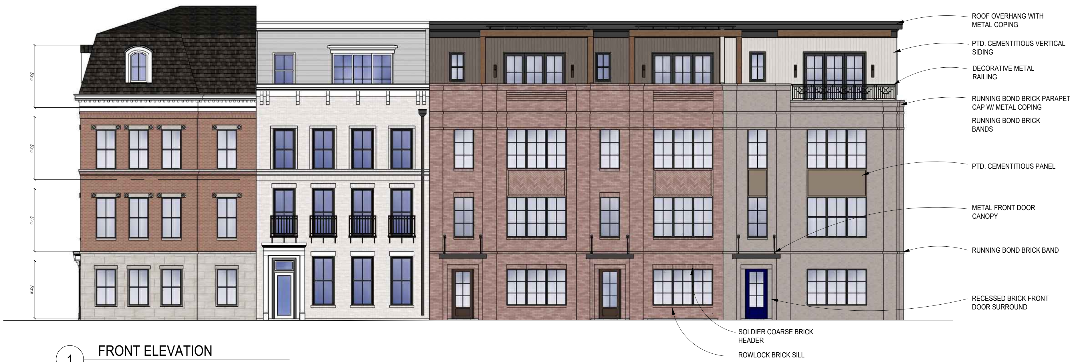
1 FRONT ELEVATION Scale: 1/8"=1'
