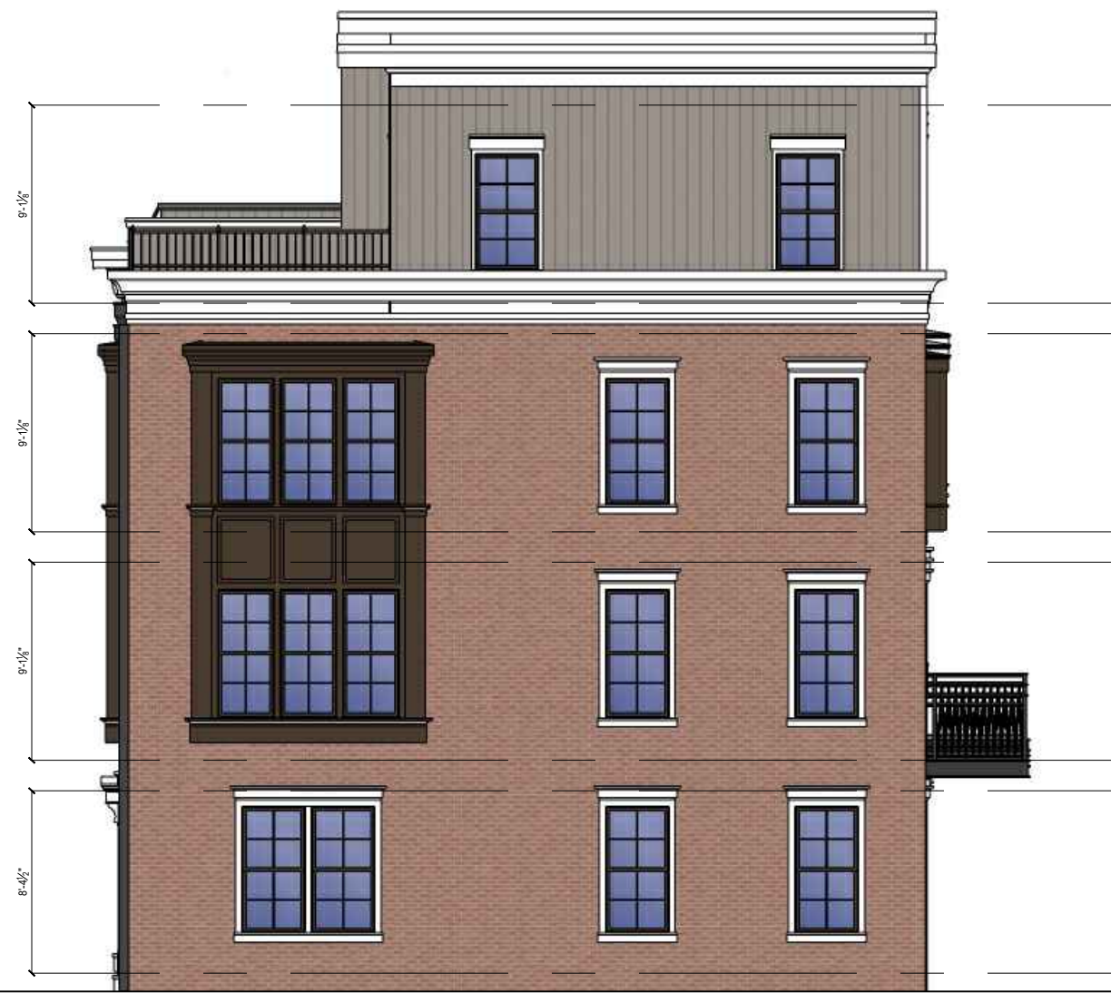
2 RIGHT SIDE ELEVATION Scale: 1/8"=1'
