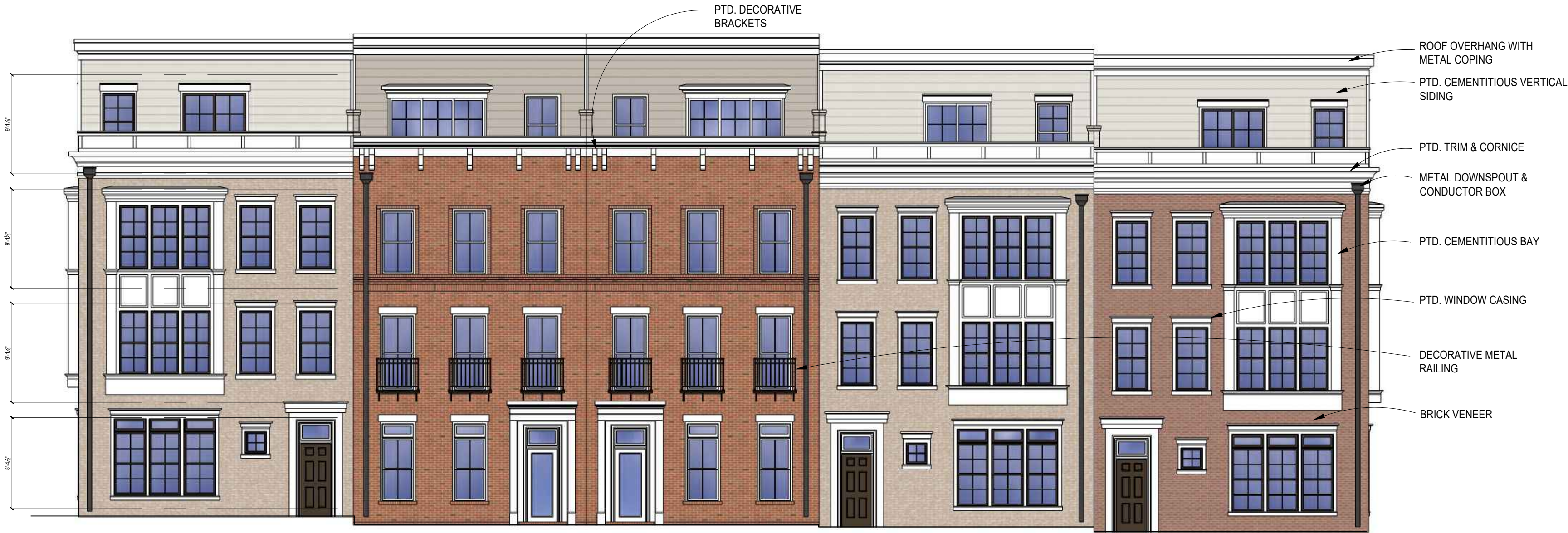
1 FRONT ELEVATION Scale: 1/8"=1'
