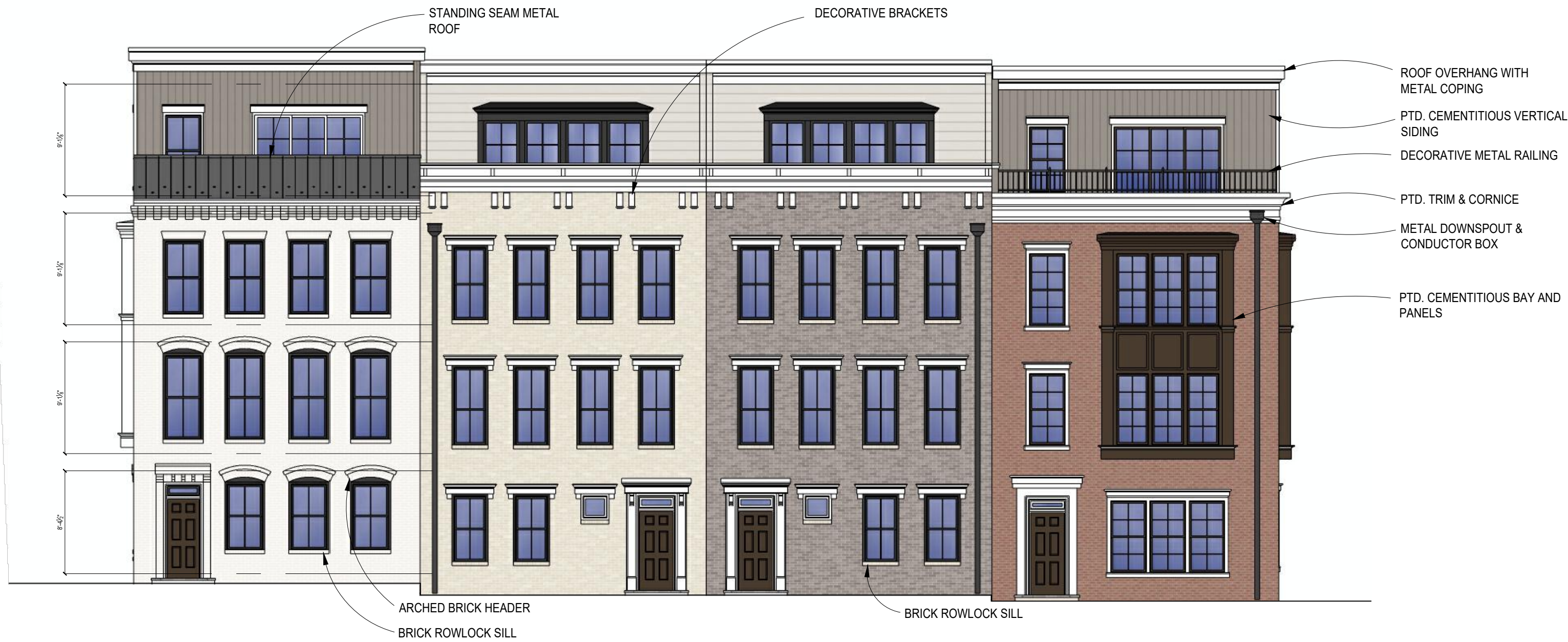
1 FRONT ELEVATION Scale: 1/8"=1'
