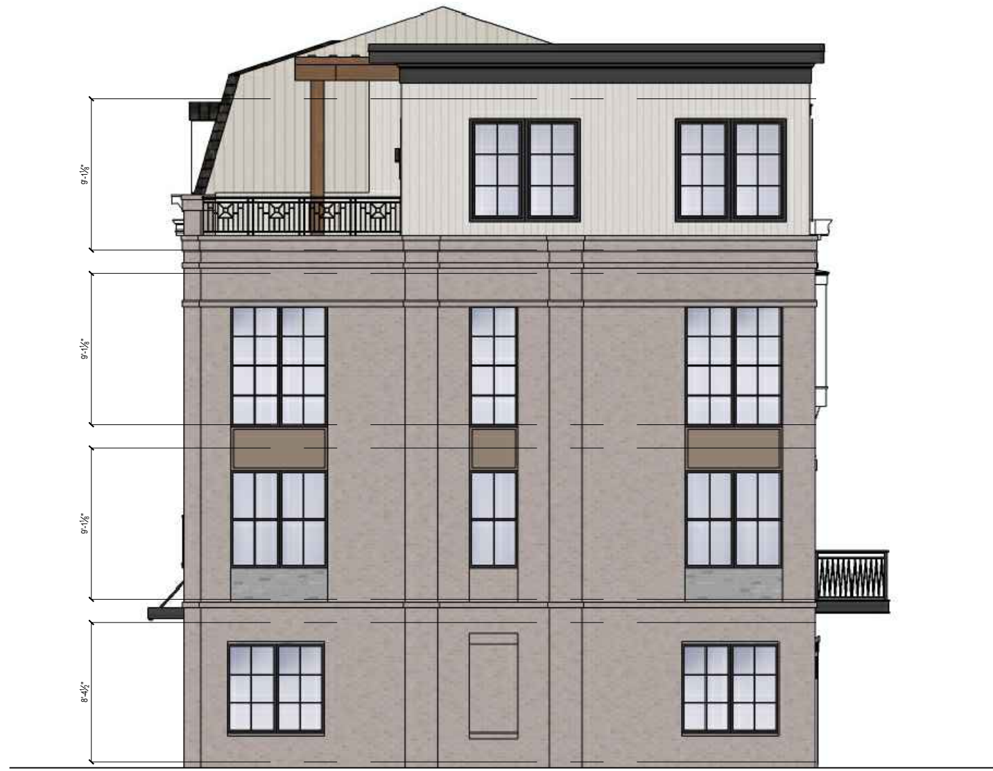
2 RIGHT SIDE ELEVATION Scale: 1/8"=1'
