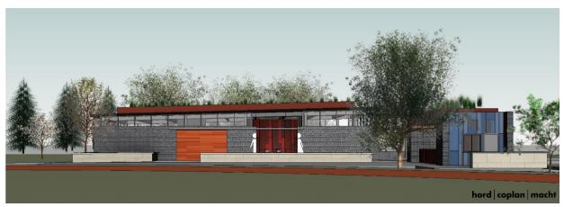
Viewed facing west: Building B (Restrooms and Storage) is gray brick. The sliding door on the left encloses the restroom entry area when not in use. The vertical panels in red and blue are painted fiber cement. The end of Building A (Concessions) is on the right.
