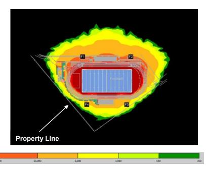
Map indicates the maximum candela an observer would see when facing the brightest light source from any direction.
