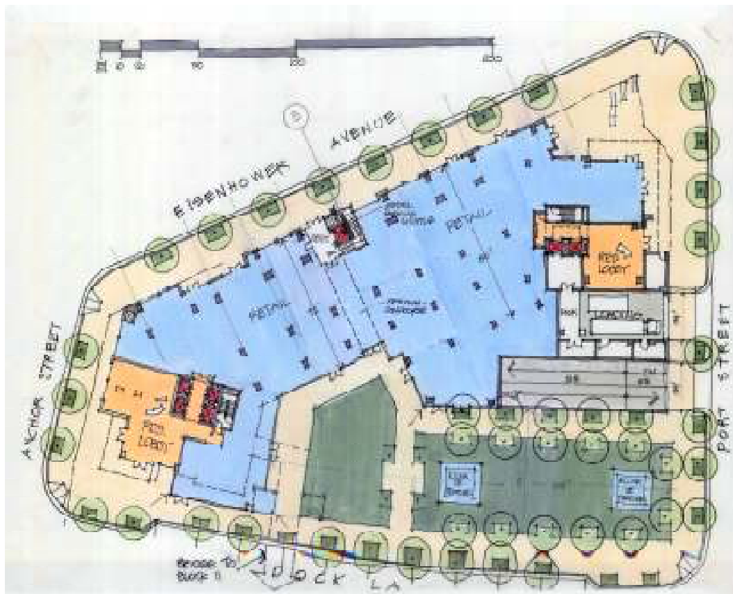
Illustrative F: Staff Alternate Ground Floor Plan - Expanded Retail Space shown in blue Note that retail elevator location gives direct access to Eisenhower Avenue and lease space.
